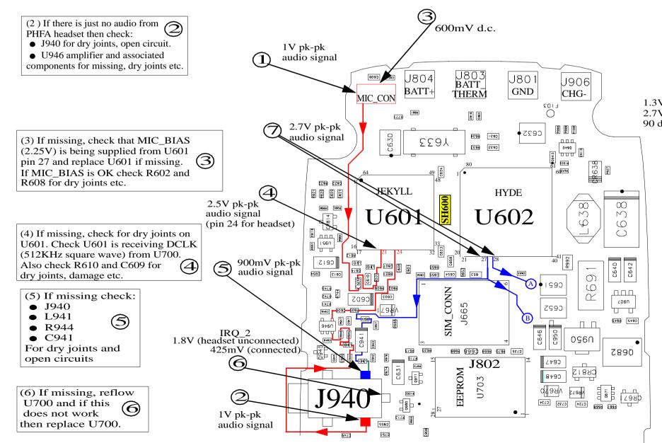
(9) If you cannot find any audio signal at any point, then this could be a data fault, check for: • DIG\_AUDIO on pins 14 and 15 U601
