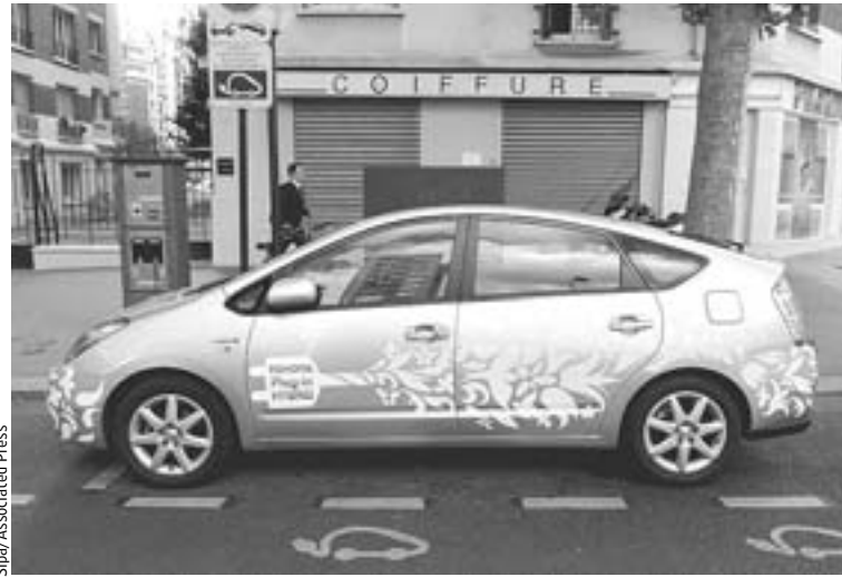
Toyota's new rechargeable Prius hybrid prototype being charged at one of Paris's charging stations.
