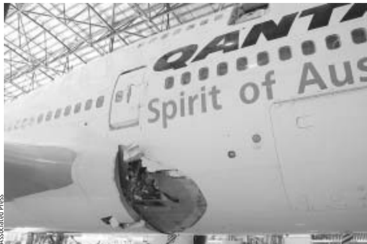
The review followed the July 25 decompression of an international flight after an exploding oxygen cylinder ripped a hole in the 747's fuselage.
