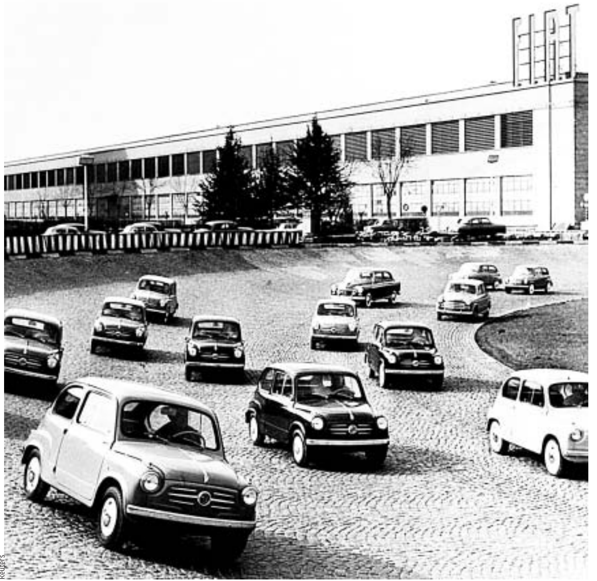
In this photo from 1955, Fiat 600s are driven on the roof track of the Lingotto factory in Turin. Like the car maker that calls it home, Turin, more than any other Italian city, mixes old with new, tradition with innovation.
