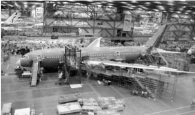
Airlines start paying for planes as they get built. Here, Boeing 787 Dreamliners undergo final assembly at the company's plant in Everett, Washington.
