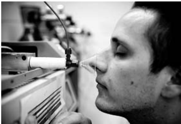
The chromatographe, a tasting machine used by beer chemists in a Belgium laboratory, allows them to sniff all the aromas of a beer with great precision.
