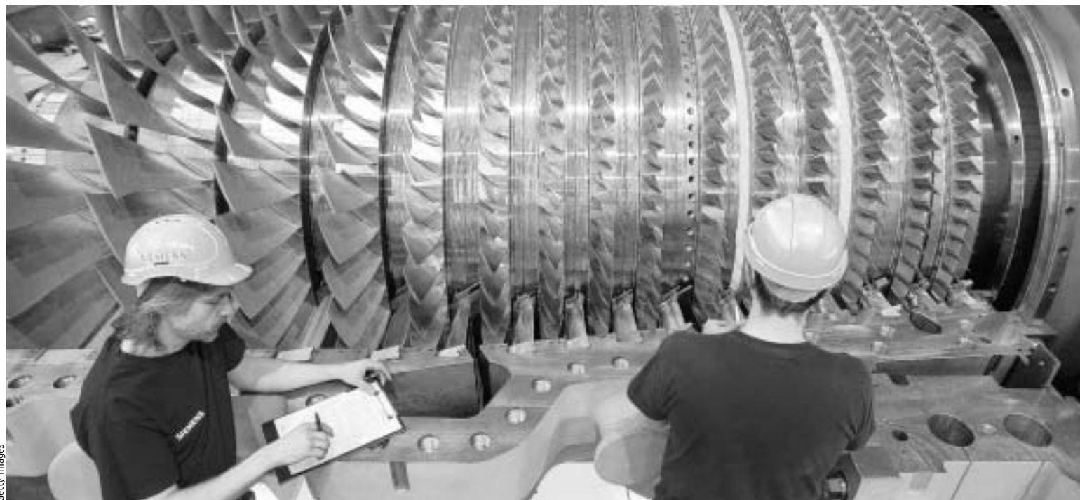
Workers assemble a gas turbine at a Siemens factory in Berlin last week.
