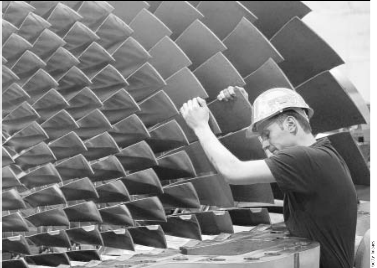
A worker rotates a gas turbine during assembly at the Siemens factory in Berlin.
