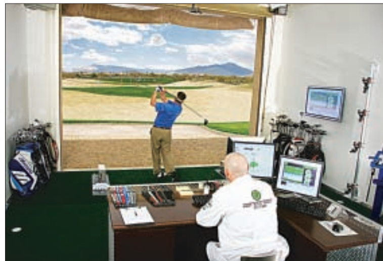
Gathering customer's 'Swing DNA' using data collected on a launch monitor that inputs it into proprietary software. Doppler radar tracks the ball and enters data in computer.
