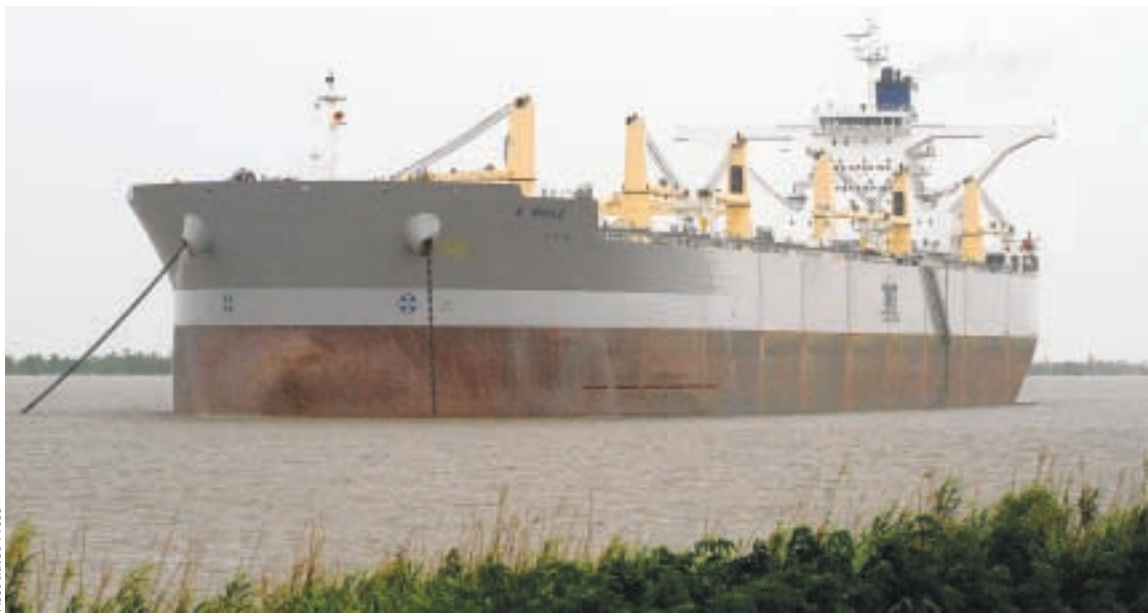
The A Whale, anchored on the Mississippi River last week, is designed to filter some 500,000 barrels of oily water a day.
