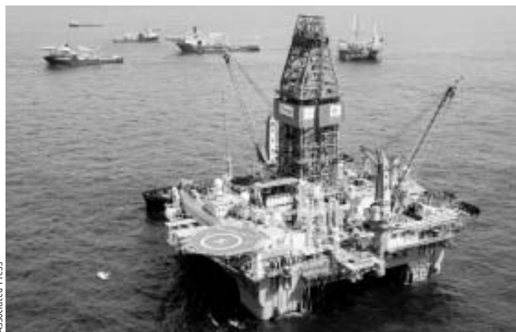
A rig drills a relief well at the site of the Deepwater Horizon in August.
