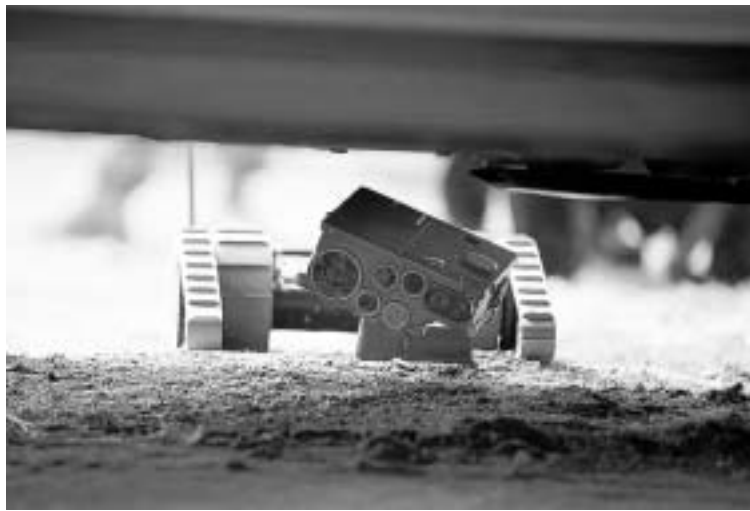
Clockwise from top: Specialist Joshua Gabbard tests a Small Unmanned Ground Vehicle (SUGV), intended for reconnaissance operations in buildings or at vehicle checkpoints; soldiers prepare to fly a Class I Unmanned Aerial System for reconnaissance, surveillance and target acquisition, which can fly up to eight kilometers from the operator and then be handed off to a remote operator in closer range; the SUGV gets a closer look at a suspicious vehicle.
